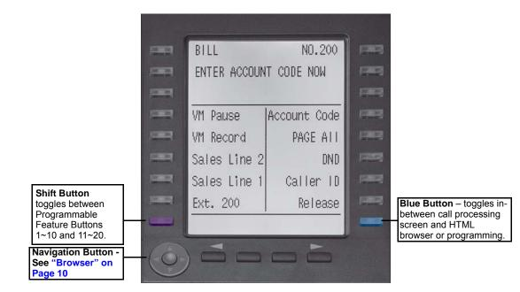
Web pages display basic HTML but do not support ASP or Flash. The 18 buttons that surround the screen can be used to highlight selections in the browser. The Navigation Button can be used to move the viewing window across the website; the center of the navigation button can be pressed to select a field that is highlighted.
